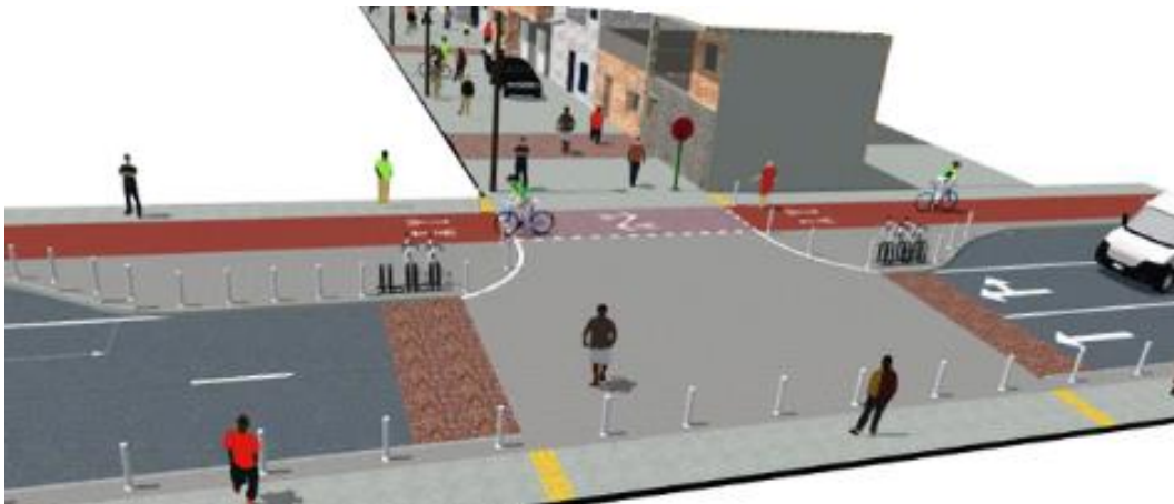
Figure 3.12. Extension of curbs towards the road.
