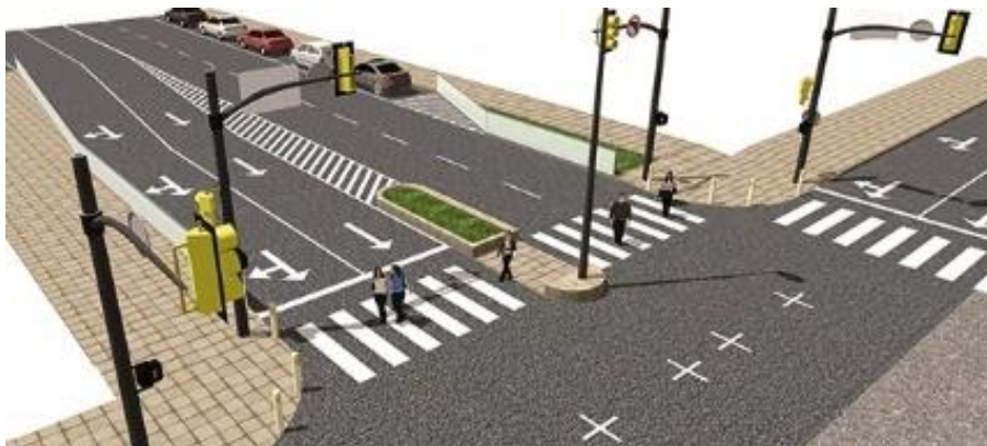
Figure 3.16. Arrangement of a median island as refuge for pedestrians.
