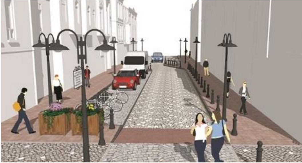
Figure 3.17. Proper arrangement of the sidewalk – delimited by the areas where vehicles can be parked.
