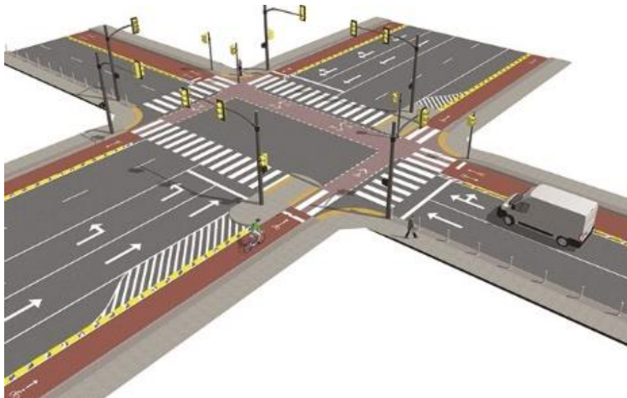
Figure 3.17. Arrangement of a traffic light intersection with controlled signal.
