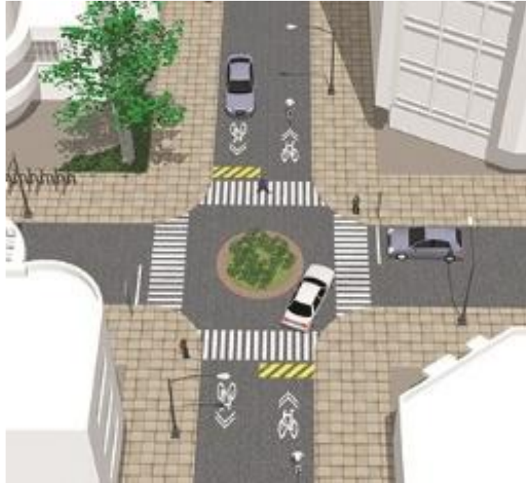
Figure 3.14. Arrangement of central islands in intersections.
