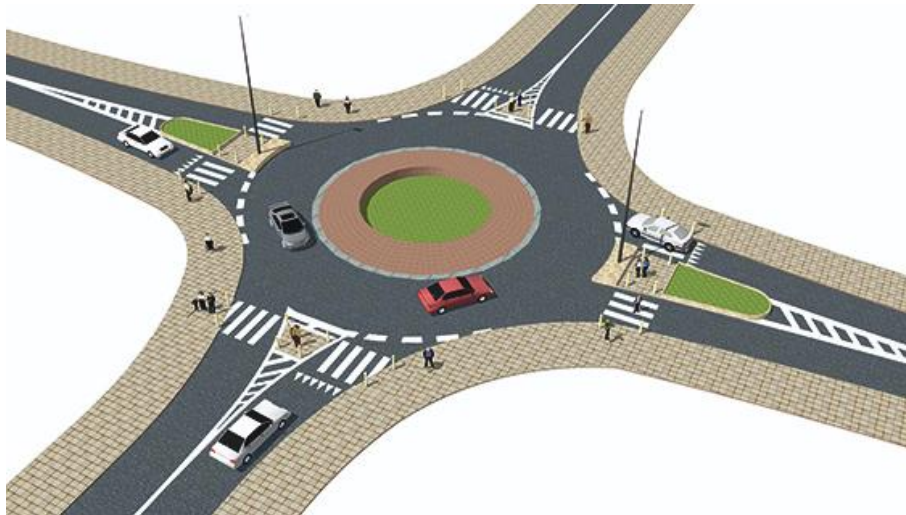
Figure 3.15. The arrangement of a roundabout.
